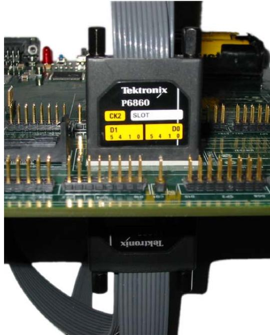
**PCB with back-to-back P6860 probes installed**
