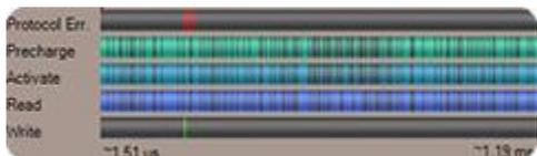
These products also come with the [NEX-DDR-PROTOCOL](#) software tool. This software provides statistical information and global bus activity to quickly give the user an overview of the DDR3 bus activity without having to revert to a listing or
