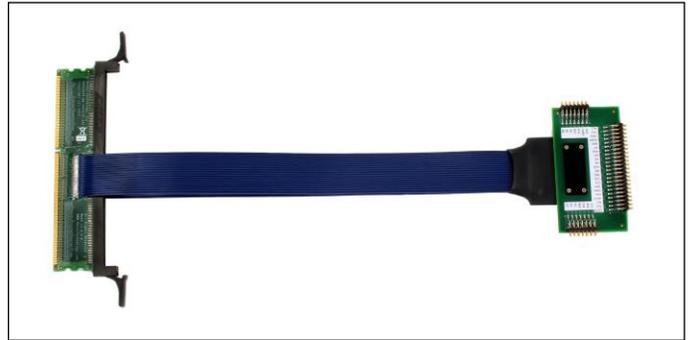
Nexus Technology recommends DDR3 slot interposers for applications where the customer must have the greatest flexibility in the probing of different DDR3 DIMMs.
