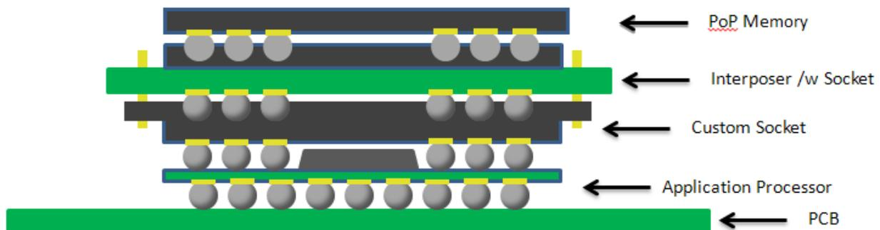
Figure 3 - Side view of the complete interposer installation
