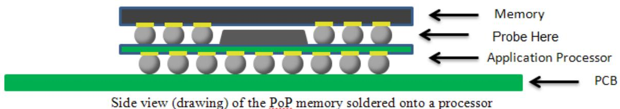
Side view (drawing) of the PoP memory soldered onto a processor
