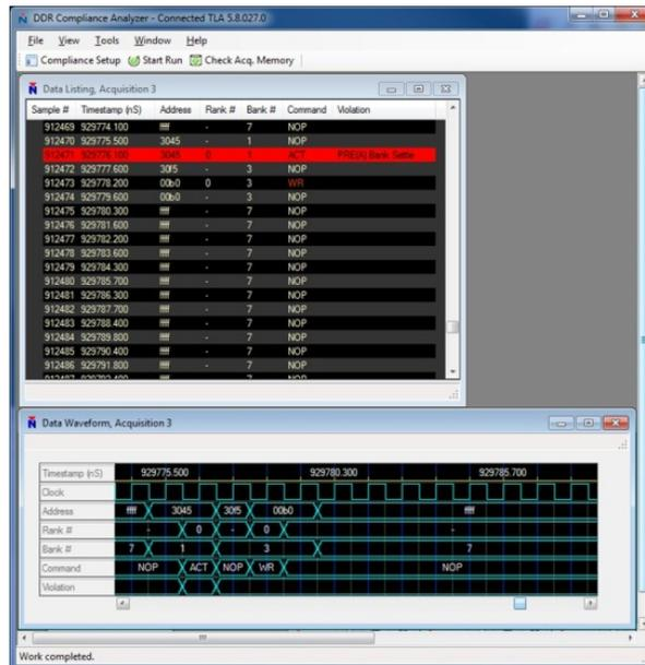
Figure 12 - Waveform & Timing Displays of Compliance Analysis
