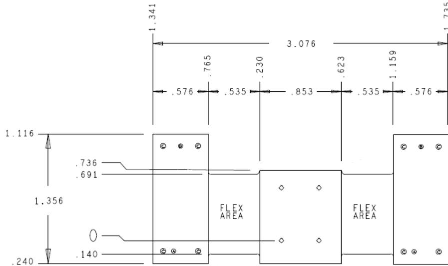
Figure 17 - LPDDR2 168 – ball /4Logic Analyzer Component Interposer Dimensions
