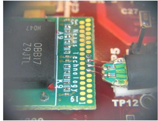
Figure 5 - Soldered down probe tips
