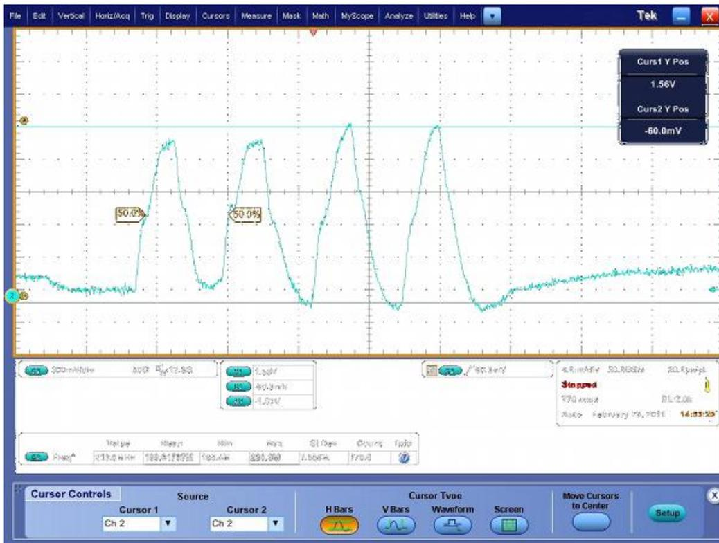
Figure 6: Strobe as seen using the Oscilloscope Component Interposer
