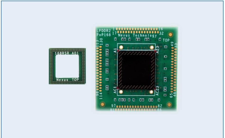
This Memory Component Interposer (MCI) BGA adapter has been designed to provide a high fidelity, easy to probe adapter that connects between your target Board and your memory component. Memory Component Interposers compliment the oscilloscope adapters providing a complete debug solution.
