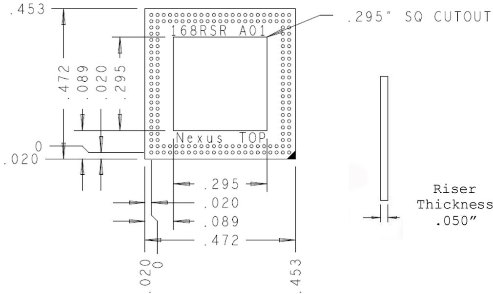
Figure 7: LPDDR2-168 ball Riser Dimensions
