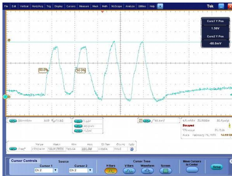
Figure 1: Strobe as seen using an oscilloscope component interposer
