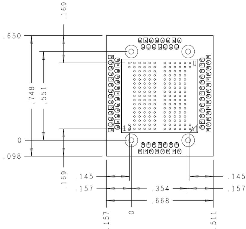
Figure 2: LPDDR3 178-Ball FBGA Oscilloscope Component Interposer Dimensions
