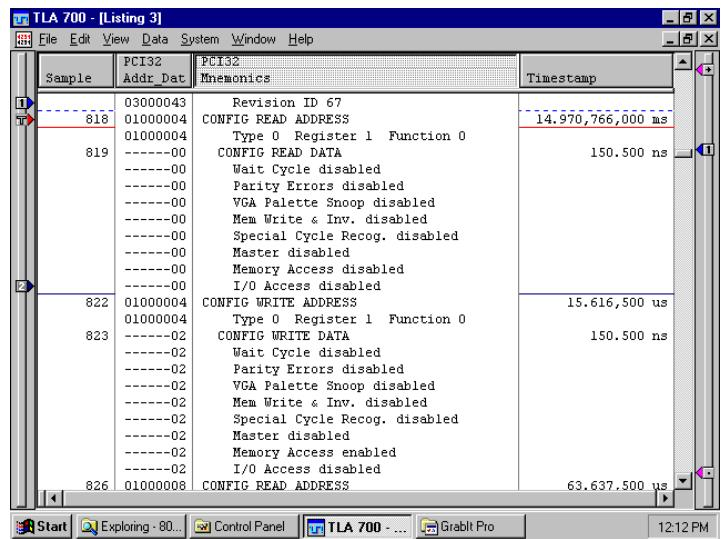
Same disassembly display with Memory and I/O cycles suppressed.
