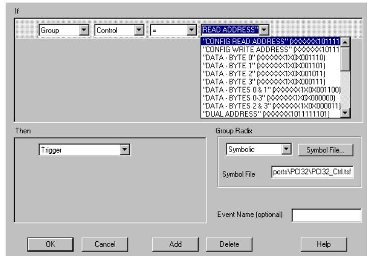
Trigger on pre-defined PCI cycles
