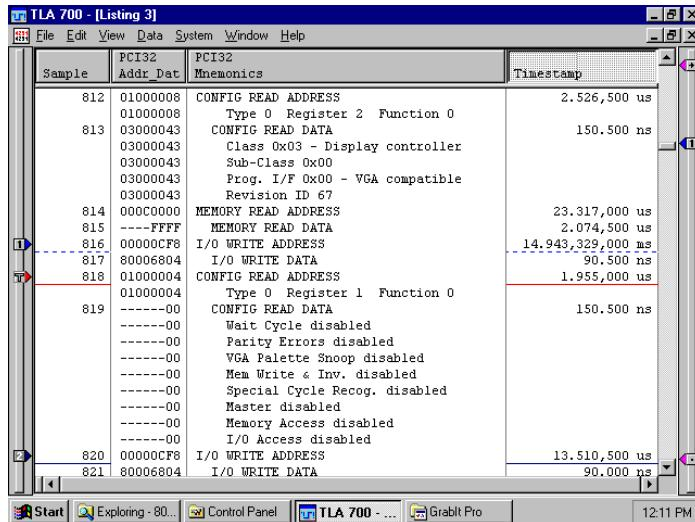
PCI cycles are identified and Config cycles are decoded. Device information is translated according to Class, sub-Class, and Type.
