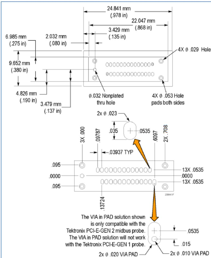
Figure 10 NEX-PRB8-SM Probe Footprint Dimensions and Keep Out Area
