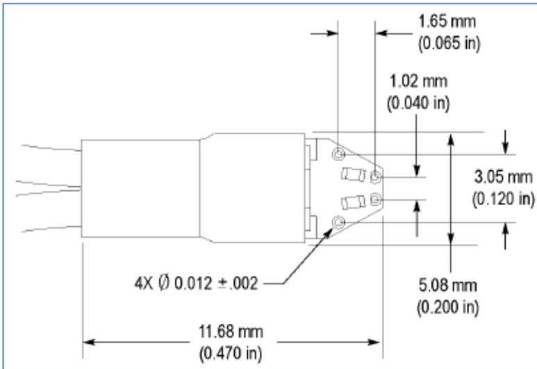
Figure 11 NEX-PRB1-SD Single Channel Serial Probe Dimensions
