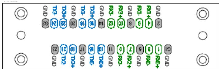
Figure 7 NEX-PRB8-SM 8ch Midbus Pin Assignments
