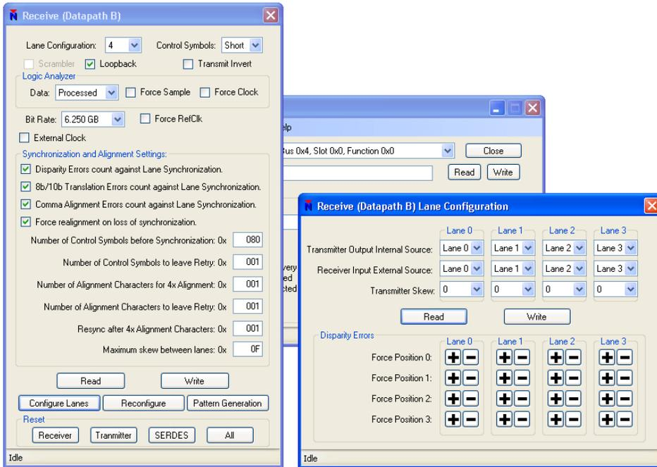
Figure 5 Configuration Interface Details
