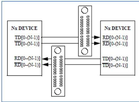
Figure 8 Recommended Midbus Probing
