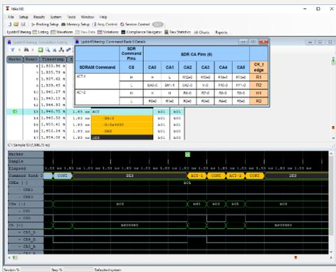
Figure 2 LPDDR4 State, Waveform and Details Example
